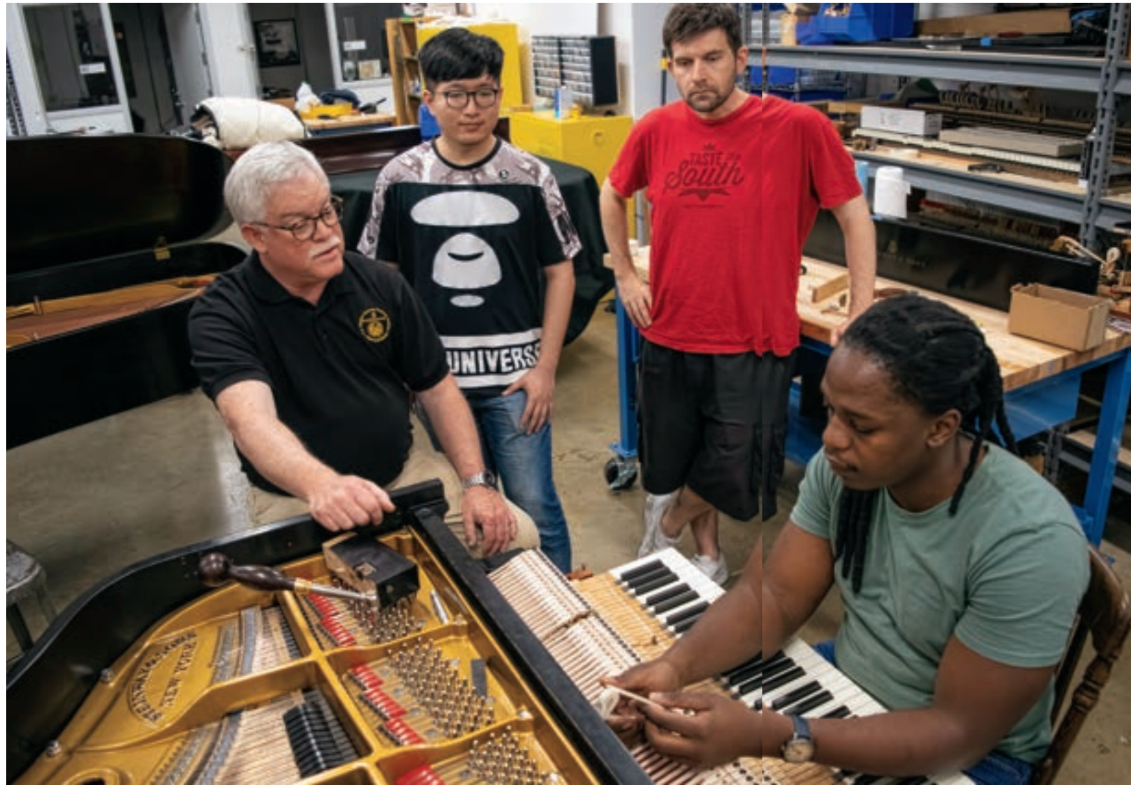
With the action removed from the piano, John Cavanaugh, left, guides Tshepiso Ledwaba and two classmates in a hammer felt resurfacing technique using a sandpaper file.
