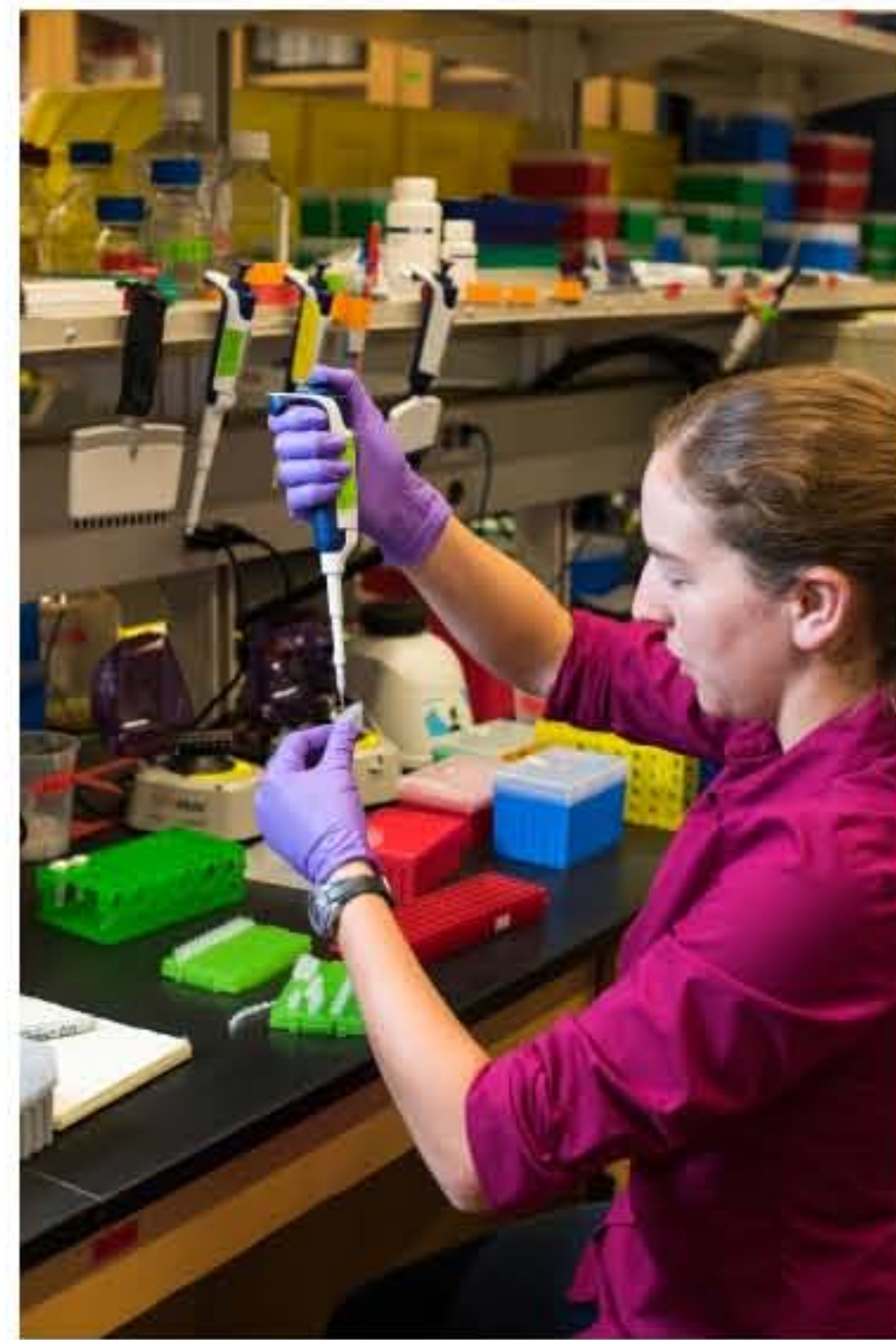
Lee Organick, a UW computer science and engineering research scientist, mixes DNA samples for storage. Each tube contains a digital file, which might be a picture of a cat or a Tchaikovsky symphony. Tara Brown Photography/ University of Washington
